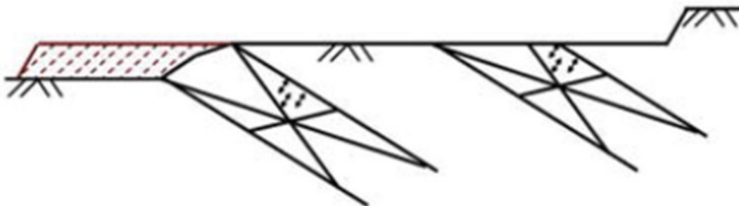
(b) Leveling the whole site of the temple foundation by excavation and backfilling
